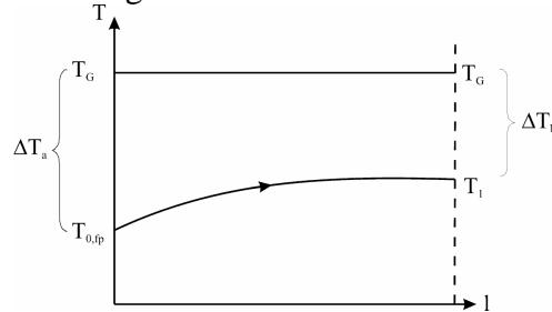
**Although the feed is of 100°C, the dilute solution reaches its bubble point in the evaporator almost at once. Therefore the boiling point is to be applied at calculating the logarithmic mean approach temperature.**
